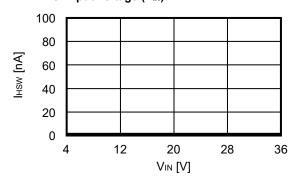
1. 11 Low side power MOS FET leakage current (I<sub>LSW</sub>) vs. Input voltage (V<sub>IN</sub>)
