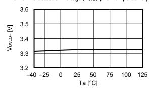
2. 7 UVLO release voltage (VuvLO+) vs. Temperature (Ta)
