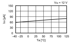
2. 2 Current consumption during shutdown (Isss) vs. Temperature (Ta)
