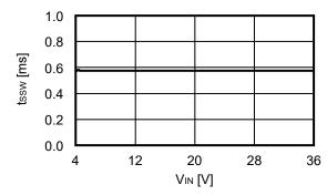
1. 7 Soft-start time (t<sub>SS</sub>) vs. Input voltage (V<sub>IN</sub>)
