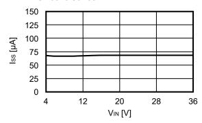
1. 2 Current consumption during shutdown ( $I_{SSS}$ ) vs. Input voltage ( $V_{IN}$ )
