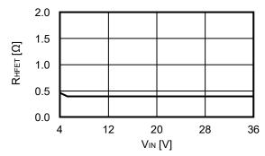
1. 9 Low side power MOS FET on-resistance (R<sub>LFET</sub>) vs. Input voltage (V<sub>IN</sub>)
