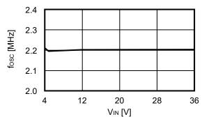
1. 5 Oscillation frequency modulation rate ( $F_{SSS}$ ) vs. Input voltage ( $V_{IN}$ )
