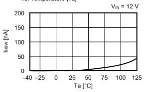
2. 13 Low side power MOS FET leakage current (I<sub>LSW</sub>) vs. Temperature (Ta)
