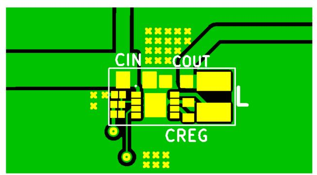
Total size  $9.0 \text{ mm} \times 4.1 \text{ mm} = 36.9 \text{ mm}^2$
