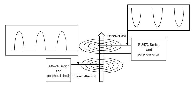
Figure 2 Reversed-phase Coil Voltage Waveform (Recommended Example)
