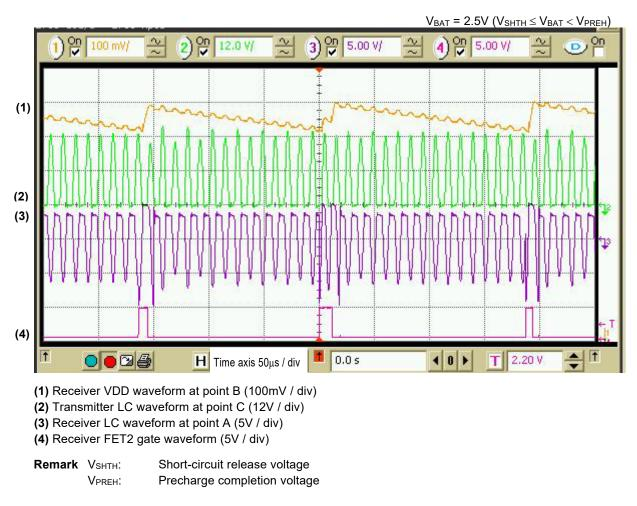
Figure 7 Relation between VDD, FET2 of Receiver and LC Waveform at Point C of Transmitter (Actual Measured Waveform)
