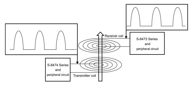
Figure 3 In-phase Coil Voltage Waveform (Non-recommended Example)
