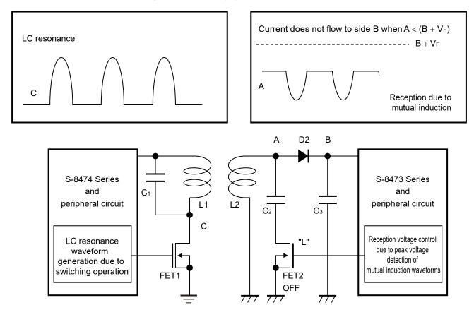
Remark V<sub>F</sub>: Forward voltage of the diode D2
