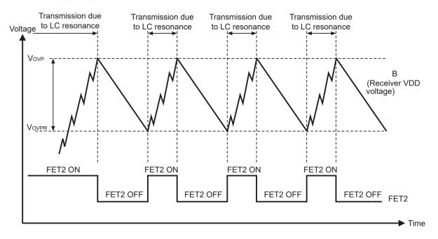
Figure 6 Relation between Receiver FET2 Control and Receiver VDD Voltage (Conceptual Diagram)
